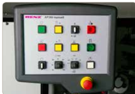
Manual control panel for setup.
